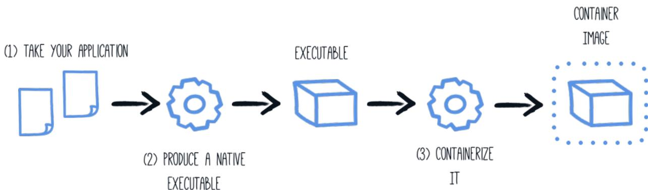
By default, the native executable is tailored for your operating system (Linux, macOS, Windows etc). Because the container may not use the same *executable* format as the one produced by your operating system, we will instruct the Maven build to produce an executable from inside a container:
